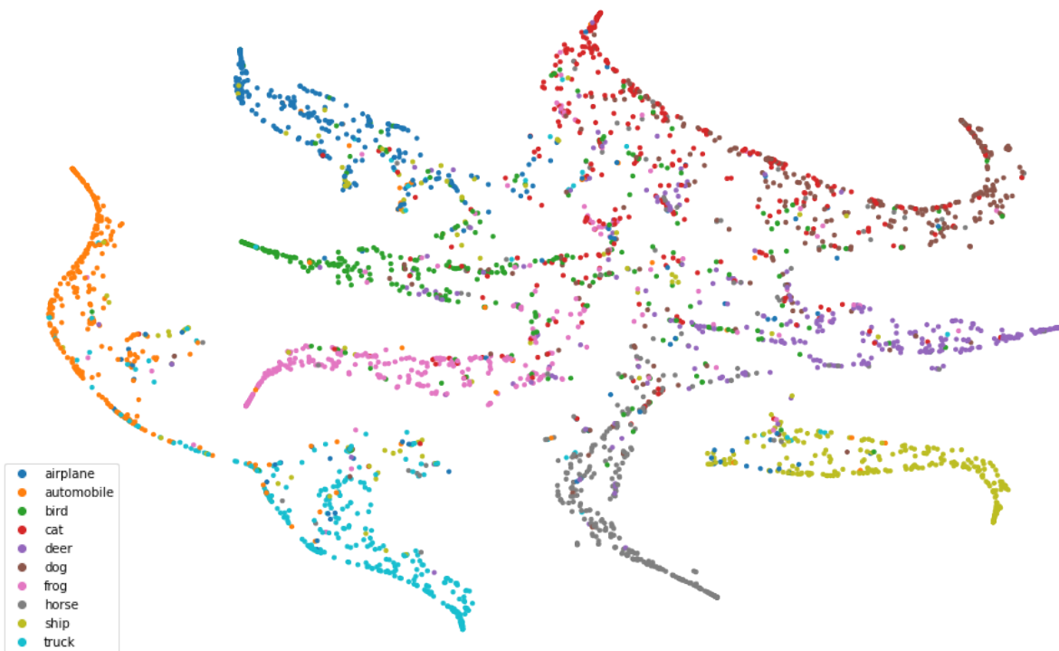
Figure 3. Clustering map using t-SNE on activation values in the final classification layer of experiment 3 showing strong clustering in all categories except cat/dog.
